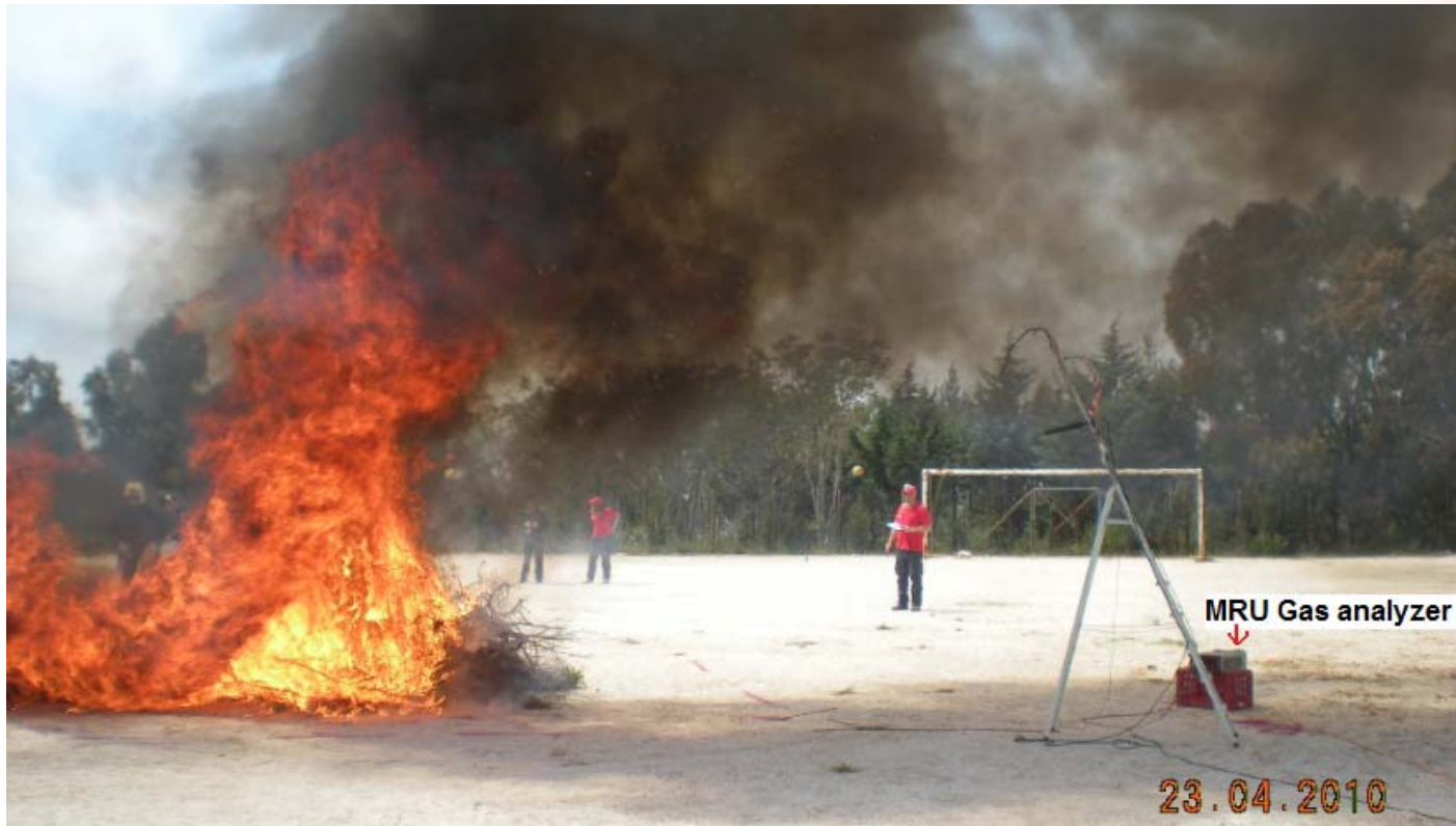
Gas analyzer measuring during the field experiment
