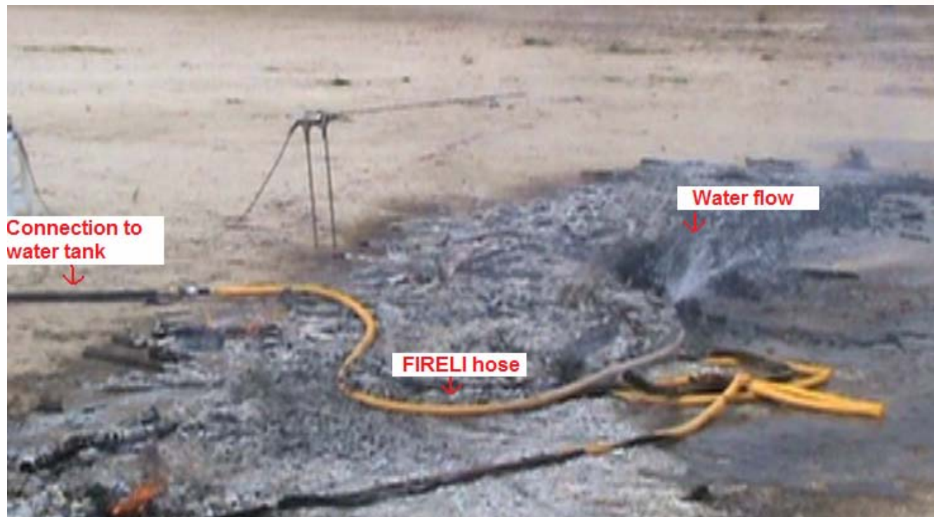
The FIRELI hose during the smoldering-glowing phases of the fire
